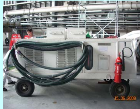
Electric power-driven mobile packaged ACU
