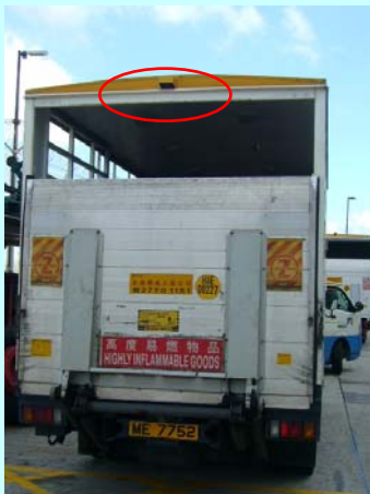
Goods truck with visual monitoring device for reversing installed
