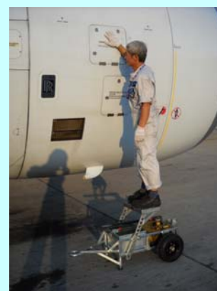
Step integrated on engine C-duct hydraulic pump
